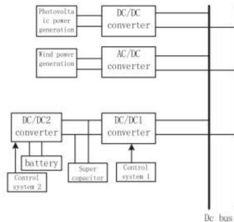
Figure 1. The improved hybrid energy storage system topology.
