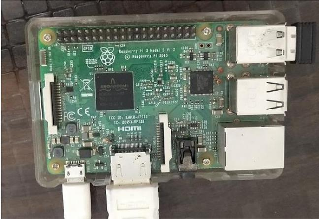
Figure 5 Raspberry Pi 3B Model
