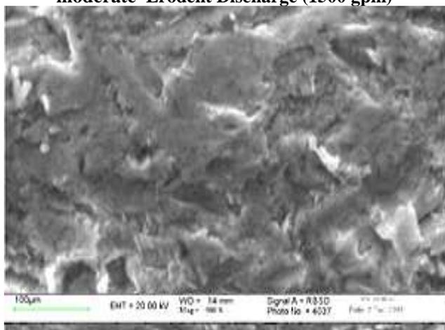
**Fig. 11(a) SEM Image of Uncoated Naval Brass at higher Erodent Discharge (2500 gpm)**
