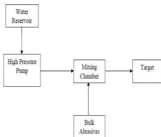
**Fig. 1 Schematic Diagram of Water Jet Erosion Test Rig**
