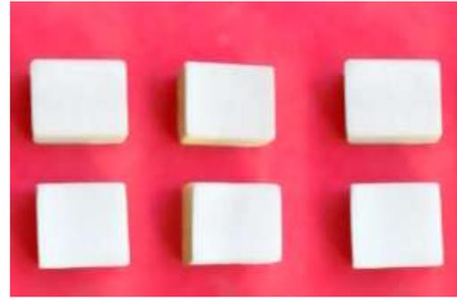
Fig. 4 HVOF Sprayed WC-Co-Cr coated naval brass
