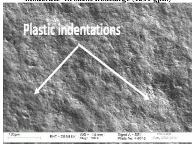
**Fig. 11(b) SEM Image of Uncoated Naval Brass at higher Erodent Discharge (2500 gpm)**
