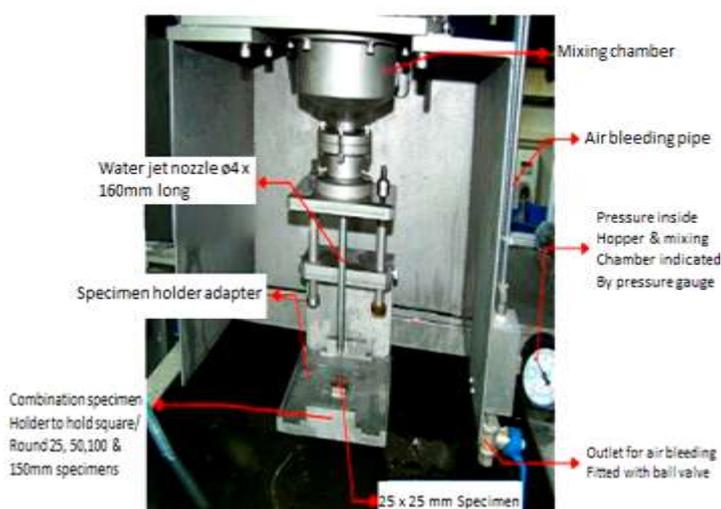
**Fig. 2 Water Jet Erosion Test Setup**
