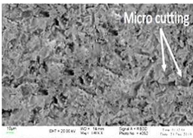
**Fig. 10(a) SEM Image of Uncoated Naval Brass at moderate Erodent Discharge (1500 gpm)**
