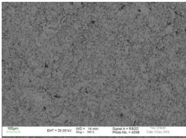
**Fig. 9(a) SEM Image of Uncoated Naval Brass at lower Erodent Discharge (500 gpm)**
