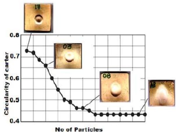
Fig. 8. Effect of Eroder Discharge on crater formation
