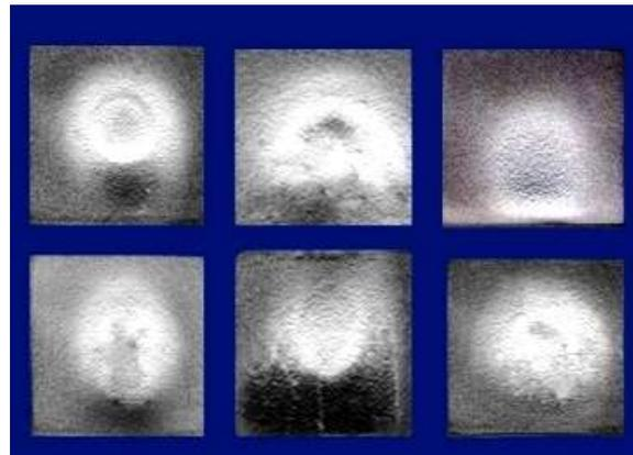
Fig. 6 Slurry Eroded Test Specimens of WC-Co-Cr Coated Naval Brass
