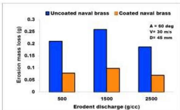
Fig. 7 Effects of Eroder Discharge on Erosion
