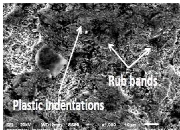
**Fig. 10(b) SEM Image of Coated Naval Brass at moderate Erodent Discharge (1500 gpm)**
