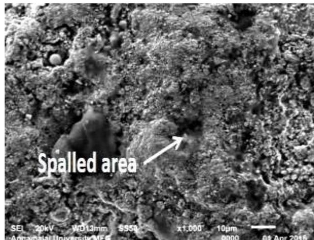
**Fig. 9(b) SEM Image of Coated Naval Brass at lower Erodent Discharge (500 gpm)**
