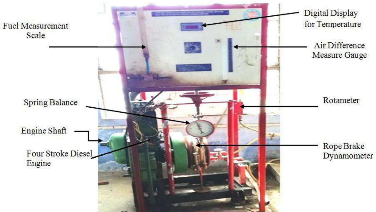
**Fig.2 Actual view of experimental setup**
