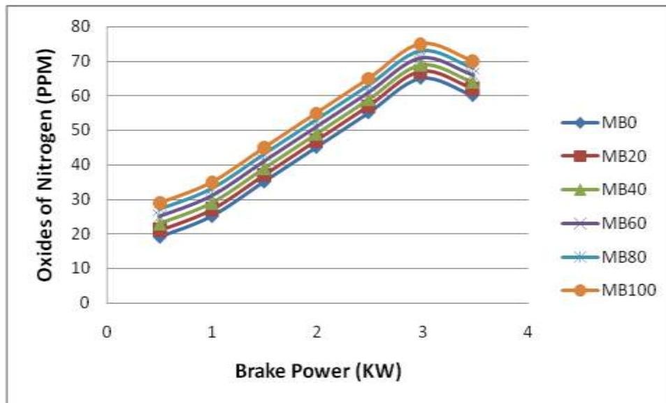
Fig. 4.6 Variation of oxides of nitrogen and brake power for different blending ratios
