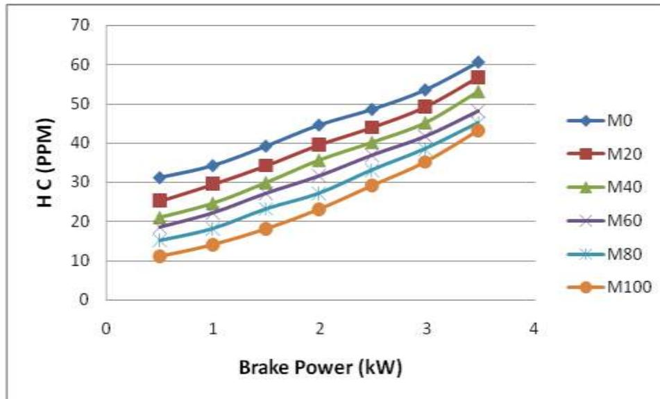
Fig. 4.5 Variation of hydro carbon and brake power for different blending ratios
