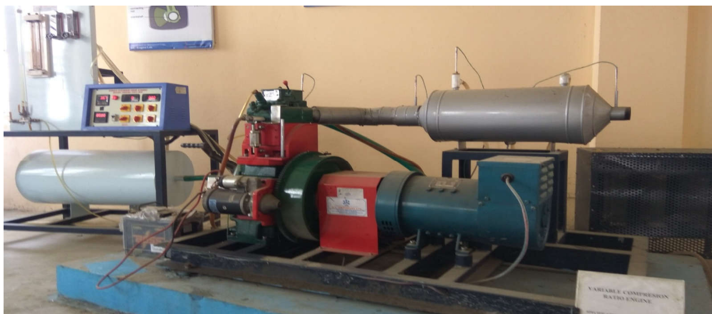
Figure 1.2 – Experimental setup and test rig of Variable Compression Engine
